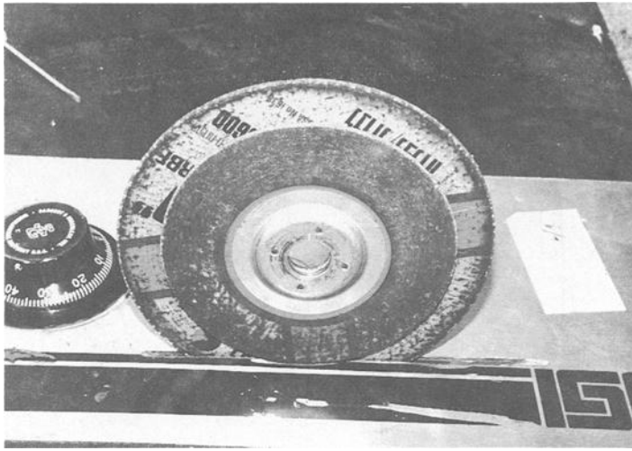
FIG. 4—The match between the combination of the two discs and the cuts in the safe door.
